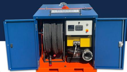
The Otter™ Mini is a hydraulically powered ultra-lightweight, high-volume, composite floating submersible pumping system capable of flows up to 2000 GPM (7571 LPM) used for remote water supply sourcing and emergency dewatering operations.
